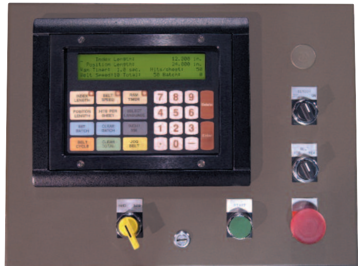
Control panel on moveable console with digital readout
